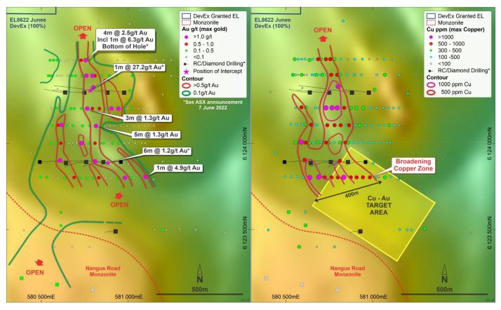
Figure 9a: Nangus Road Prospect showing location of current drill-holes. AC drilling has been thematically mapped to show maximum gold values down the hole.
