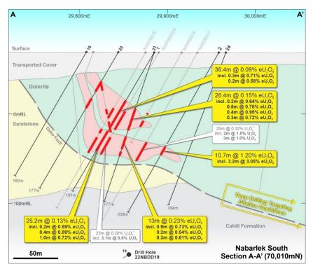
**Figure 3**: Nabarlek South – local grid cross-sections showing preliminary uranium equivalent down-hole results from DD drilling (refer to Figure 6 for drill-hole locations).
