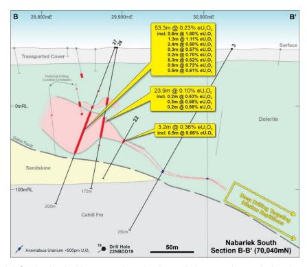
**Figure 4**: Nabarlek South – local grid cross-sections showing preliminary uranium equivalent down-hole results from DD drilling (refer to Figure 6 for drill-hole locations).
