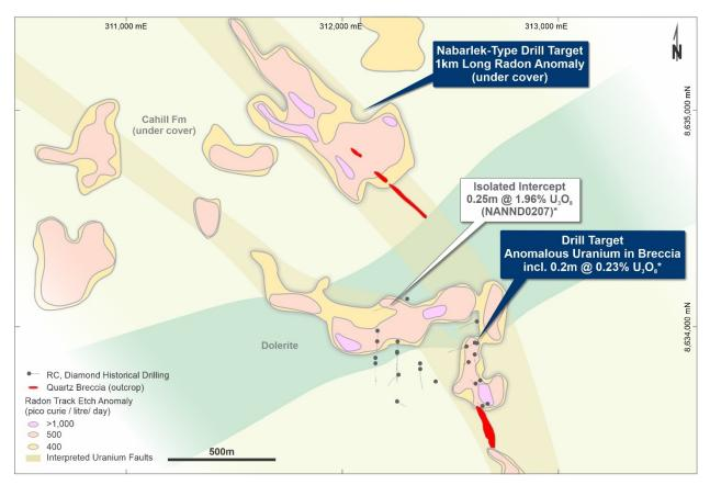
**Figure 8**: Overload Prospect – historical drilling of a uranium-bearing Nabarlek-type quartz breccia required further RC/DD drilling down-dip into more prospective lower Cahill Formation Rocks, along with testing a large radon-track etch anomaly to the north.
