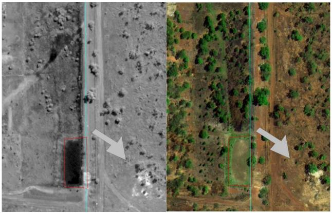
Figure 19: Plant Run-off Pond Revegetation Comparison between black and white Airphoto (2009) and colour Geo Image (2016) showing good revegetation of the area. Arrow indicates redirection of drainage leading into the pond following recontouring and filling in the pond.
