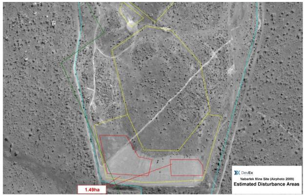
Figure 20: 2009 Airphoto of the Waste Rock Run Off Pond Area showing recent recontouring
