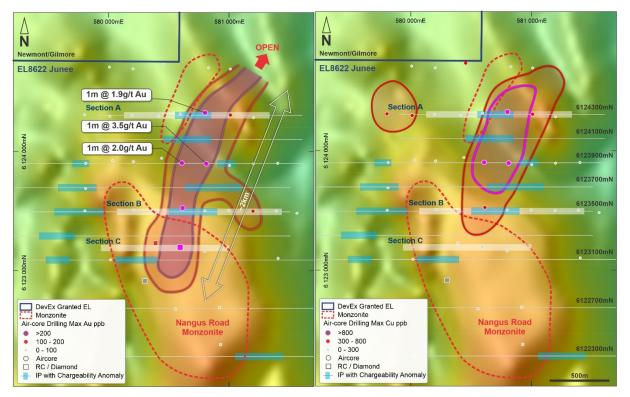
**Figure 6:** Nangus Road Prospect – Recent broad-spaced (400mN x 200mE) air-core + RC drilling, bedrock <u>copper and gold</u> <u>anomaly (maximum Au and Cu assay per hole)</u>, peak assay of 1,410ppm Cu and 3.5g/t Au (3,490ppb Au), underlain by RTP magnetics. New IP Survey lines and anomalies are also shown. The copper and gold bedrock anomaly lies within and along the northern margin of the monzonite anomaly and remains open to the north. (see Figure 7 for location).
