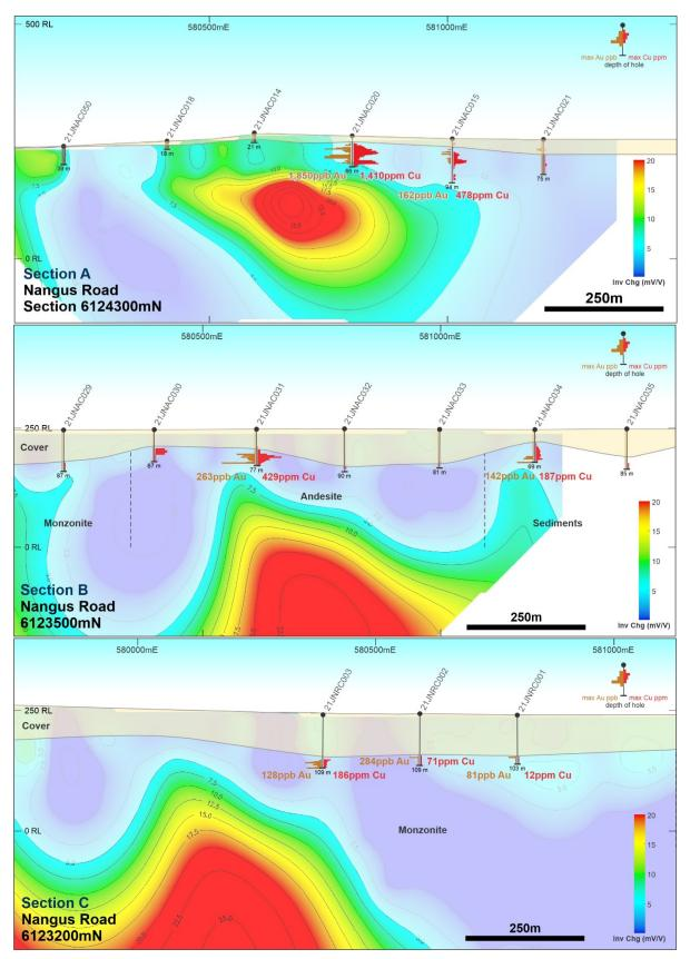
**Figure 8:** Nangus Road Prospect, Selective sections A, B and C (looking north) – showing broadly anomalous bedrock Au-Cu mineralisation overlying strong IP chargeability anomalies within and proximal to the northern margin of the Nangus Road monzonite (see Figure 2 for location).
