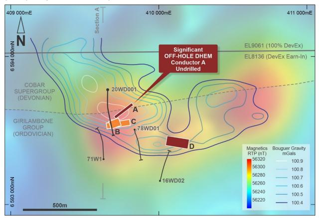
**Figure 3:** Location of modelled DHEM Conductors surrounding hole 20WD001 and the coincident RTP Airborne Magnetic image and Bouguer Gravity highs (blue contours). The coincident anomalies lie on a fault contact between the Cobar Supergroup and the older Girilambone Group – a primary exploration target horizon within the Cobar Basin.
