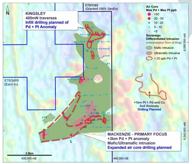
**Figure 2.** Sovereign Project: Showing the broad-spaced air-core drilling (average hole depth 25m) undertaken by DevEx last Quarter, which has defined a differentiated mafic-ultramatic intrusion with extensive elevated palladium+platinum and copper on broad traverses. The Company has recently completed an expanded air-core program to test these areas. Assays are pending.
