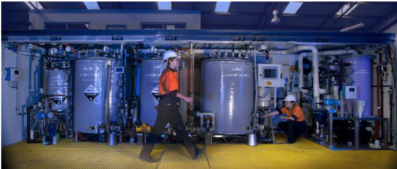
The Demonstration Plant constructed in 2011 is built inside two 40ft side opening shipping containers.
