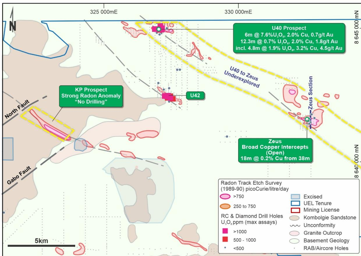
**Figure 5** – A detailed 1989-1990 Radon Track Etch survey identified priority anomalies east of Nabarlek Uranium Mine. Drilling of three of the four anomalies have identified significant uranium at U40 and U42, with significant copper seen at Zeus Prospects (see Figure 6). The KP Prospect has not be followed up and is considered a high priority target as it lies between the Gabo and North Fault and capped by the Kombolgie Sandstone.
