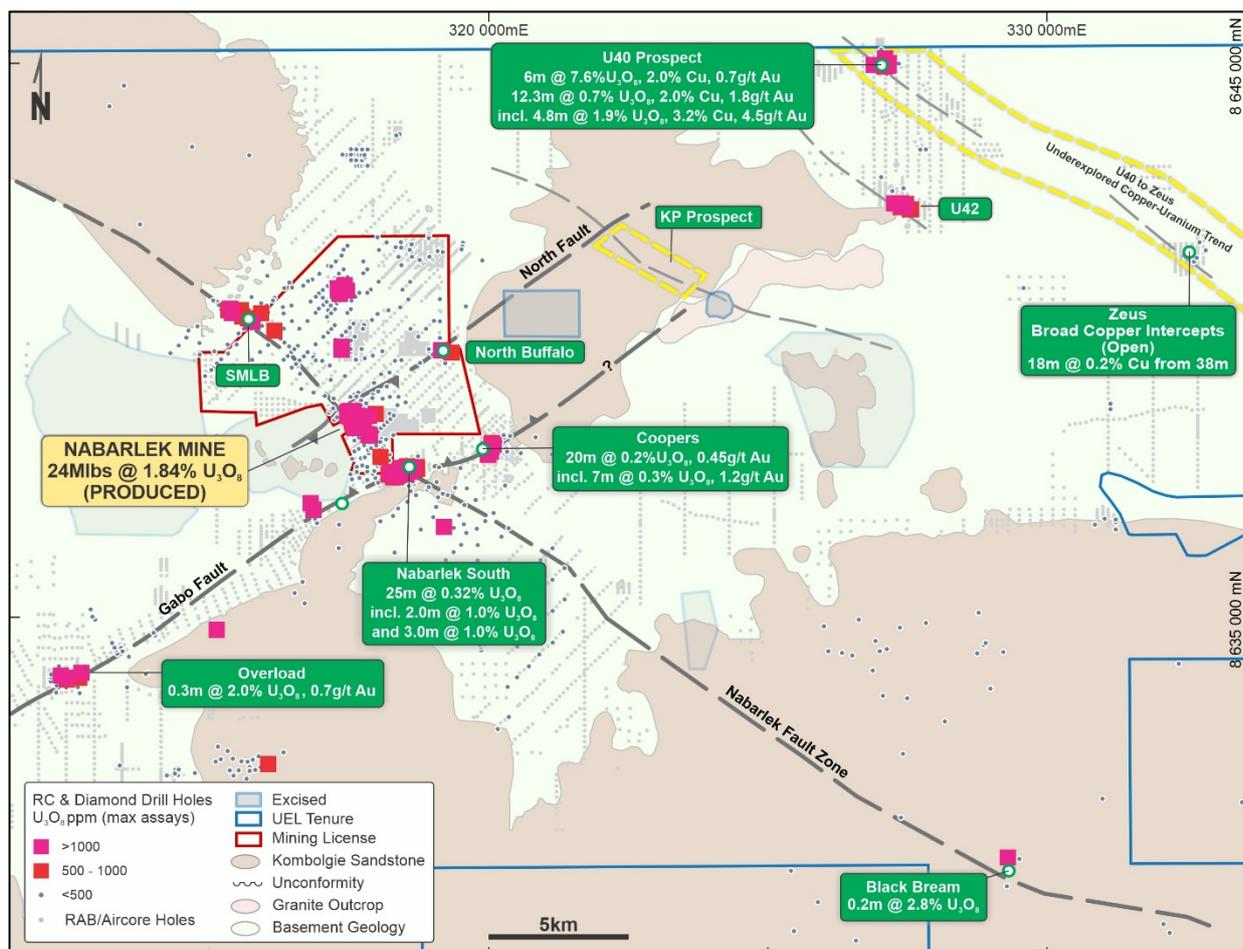
**Figure 2:** Nabarlek Project – Uranium Prospects including the historic Nabarlek Uranium Mine. Uranium-copper-gold mineralisation has been intersected within basement rocks (incl Cahill Formation and the Oepelli Dolerite) along both the Nabarlek Fault Zone (NW) and the North and Gabo Faults (NE) with the overlying Komolgie Sandstone acting as a masking cap rock to mineralisation.
