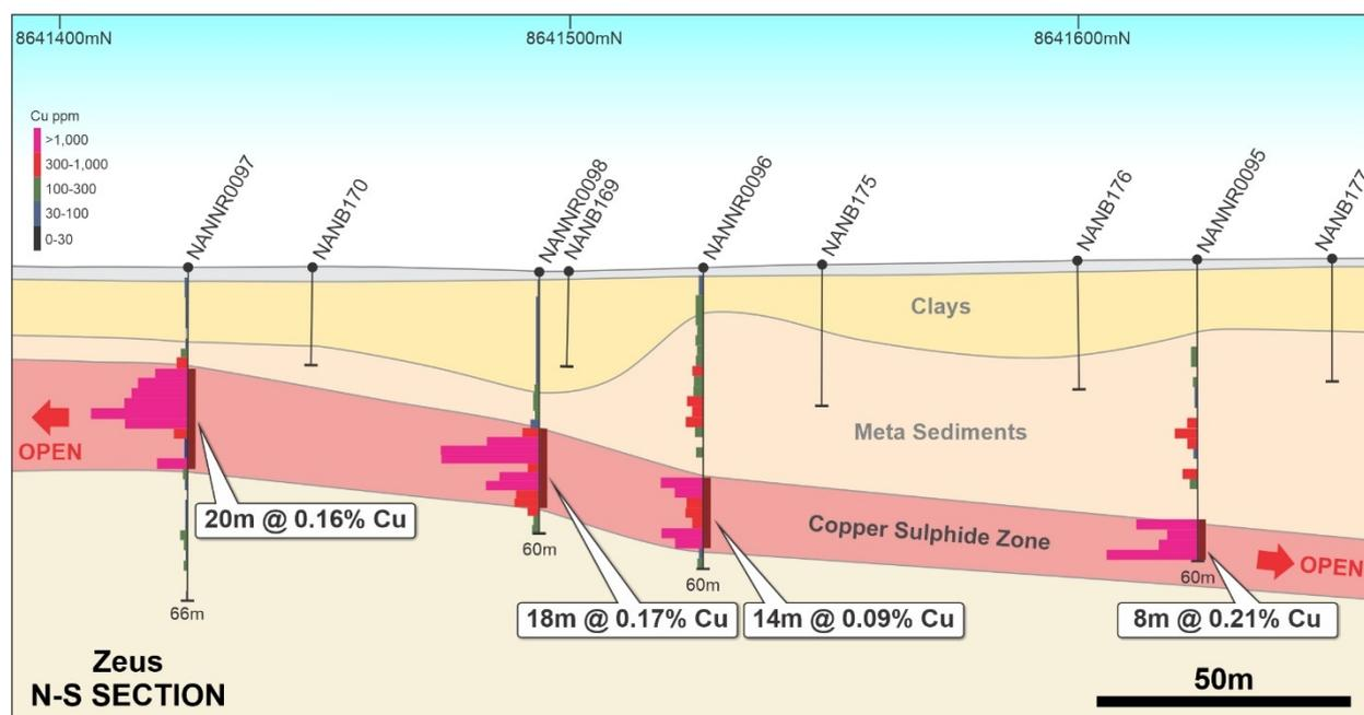
**Figure 6** – Historical 1980's Reverse Circulation drilling at the Zeus Prospect. Drilling has defined flat-lying copper mineralisation which remains open in all directions (see Figure 5). Historical RAB holes (NAB series) are also shown which were ineffective in defining the copper mineralisation.
