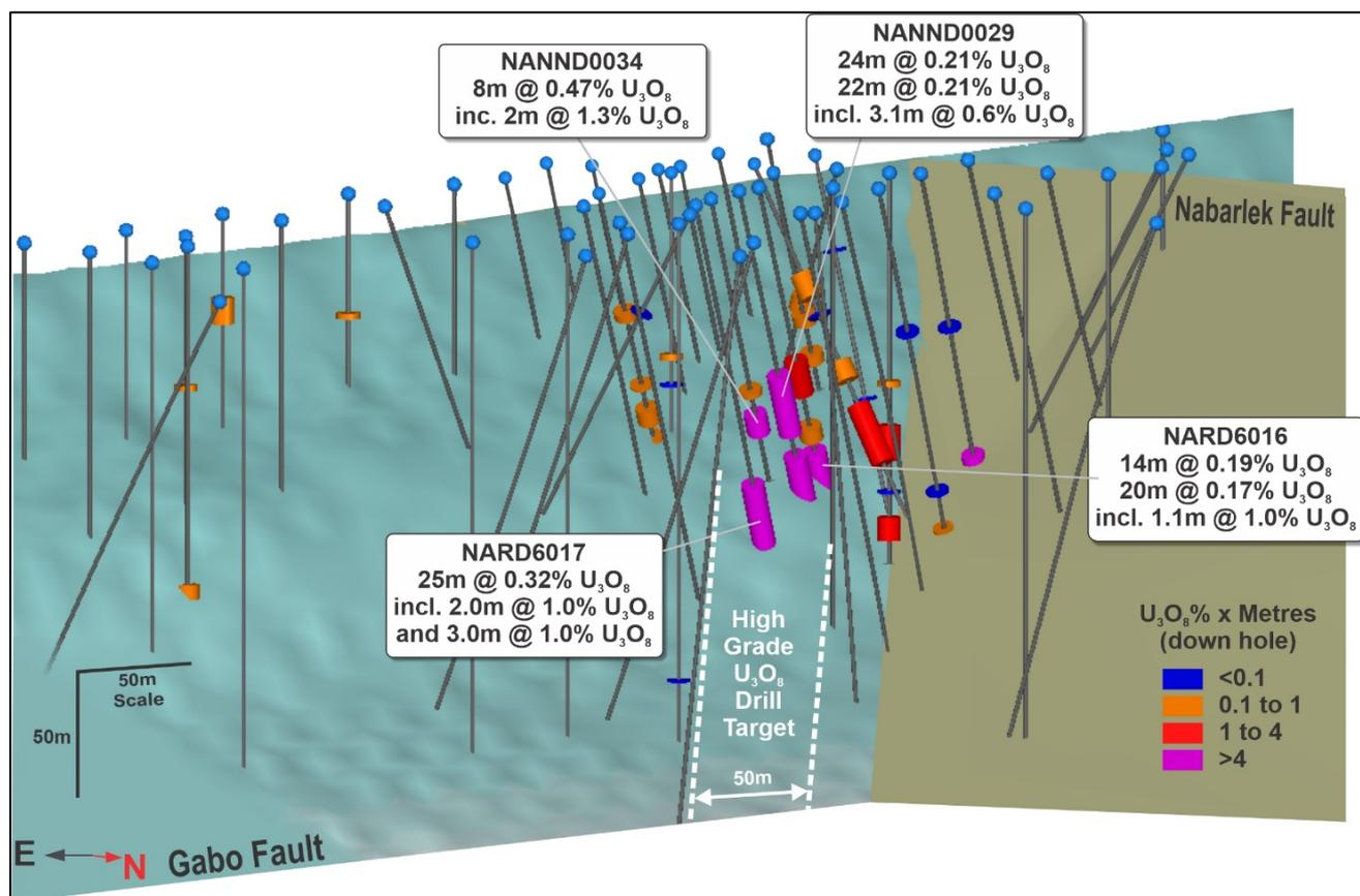
**Figure 3:** Nabarlek South – Three-dimensional view looking south-west at the intersection between the uranium-bearing Nabarlek Fault (host to the Nabarlek Uranium Mine) and the Gabo Fault. A high-grade uranium shoot is recognised to plunge to the north-east and remains open at depth.
