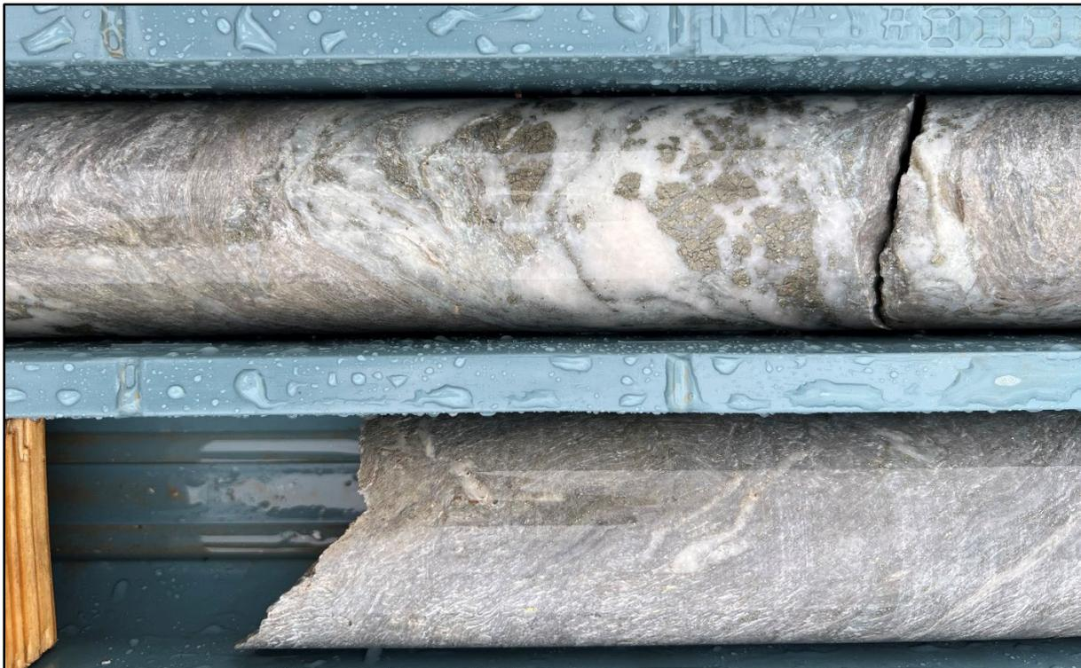
**Figure 3:** Nangus Road diamond hole 21JNDD001 close up of core at 300m (top) and 305m (bottom) showing pervasive silica, sericite, pyrite alteration with quartz pyrite veins.
