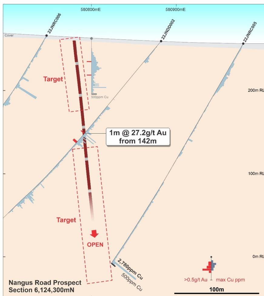
**Figure 2:** Nangus Road Cross Section (6,124,300mN) showing location of recent gold intercepts. Structural measurements from the diamond hole indicate a steep dip to the west. This zone matches well with the >1km long gold zone defined in Figure 1.
