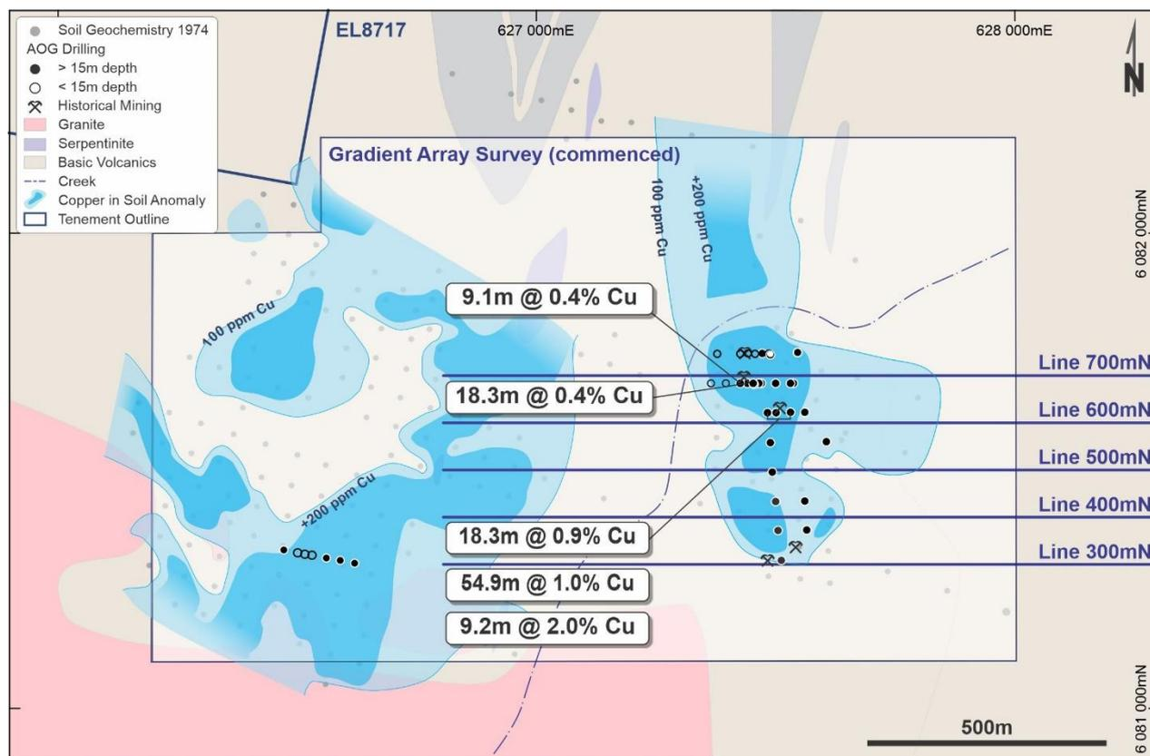
**Figure 2:** Plan View of Current IP Lines, and Gradient Array at Bogong.
