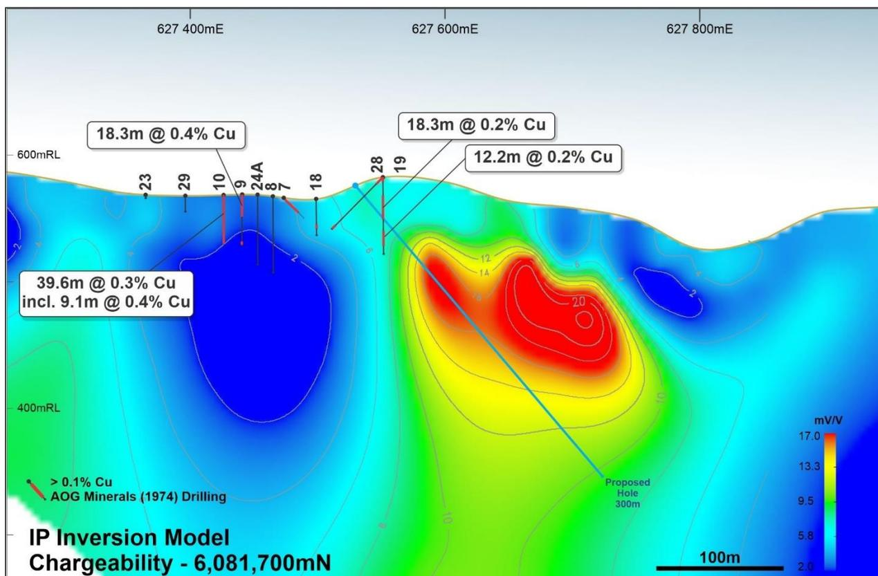
**Figure 3:** IP Inversion Model (chargeability) for line 6081700mN with historical (1974) AOG Minerals drilling and significant copper intercepts (see Appendix 2 and Company ASX Announcements on 1<sup>st</sup> August 2019 for further details of intercepts). Copper intercepts are reported as down-hole lengths as true widths are not known.
