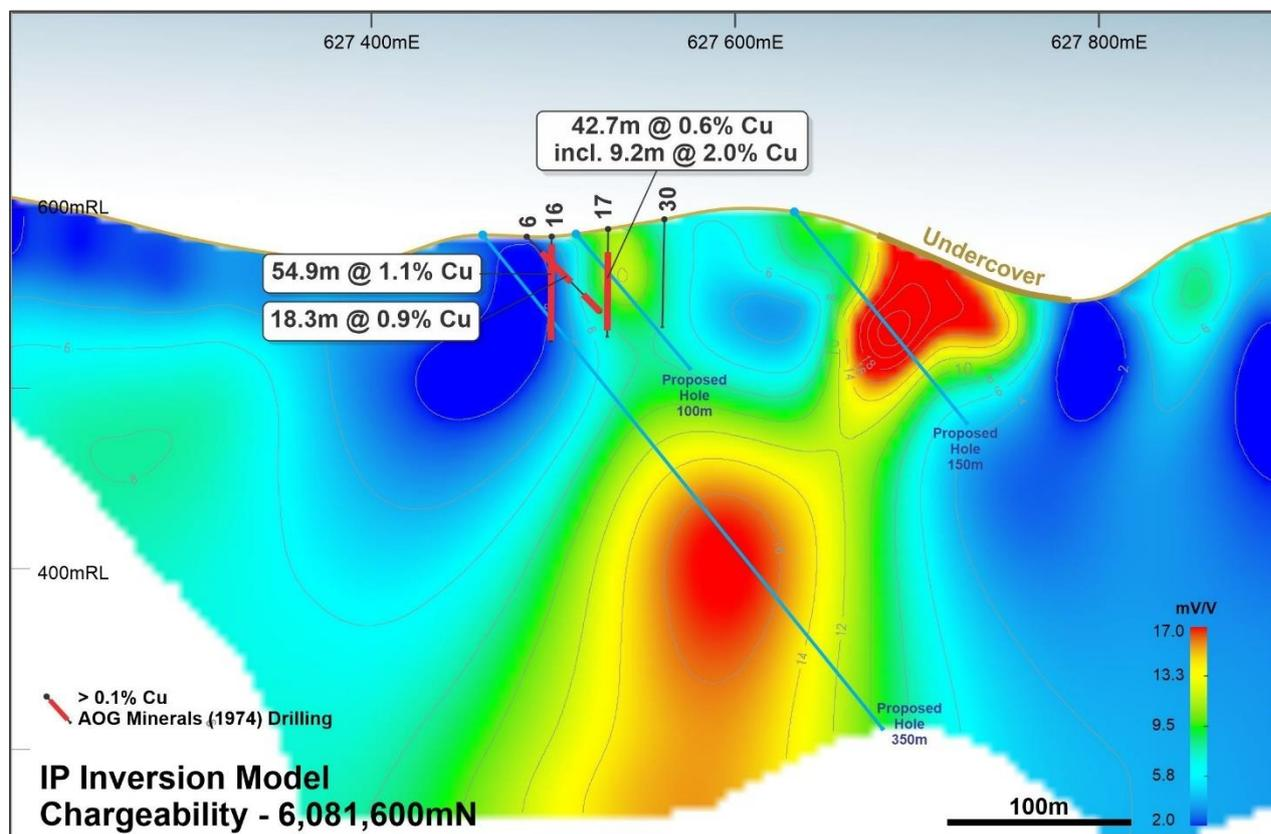
**Figure 1:** IP Inversion Model (chargeability) for line 6081600mN (line 600mN) with historical (1974) AOG Minerals drilling and significant copper intercepts (see Appendix 2 and Company ASX Announcements on 1<sup>st</sup> August 2019 for further details of intercepts). The eastern shallow chargeability anomaly is masked by soils and scree from upslope. Copper intercepts are reported as down-hole lengths as true widths are not known.
