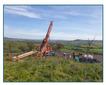
Figure 13: Diamond drill rig in operation at Junee Project, NSW.
