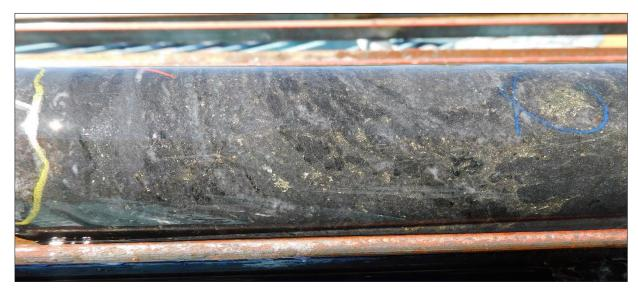
**Figure 2**: Fine-grained garnet-bearing mafic volcanic/sedimentary (country rock) near the contact of the mafic-ultramafic intrusion with copper sulphides and pyrite at 454m down-hole in Hole 2. Large garnet megacrysts (not in photo) also appears to be a focus point for copper sulphide mineralisation.
