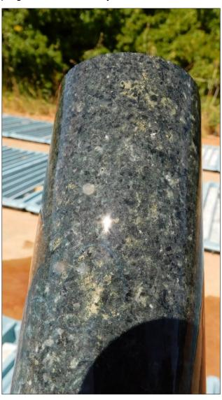
**Figure 1:** Matrix textured Fe-Ni-Cu sulphides within norite rock at 431.4m down-hole in Hole 2 (left) and disseminated Ni-Cu-Fe sulphides within norite rocks at 232.3m down-hole in Hole 2 (right).
