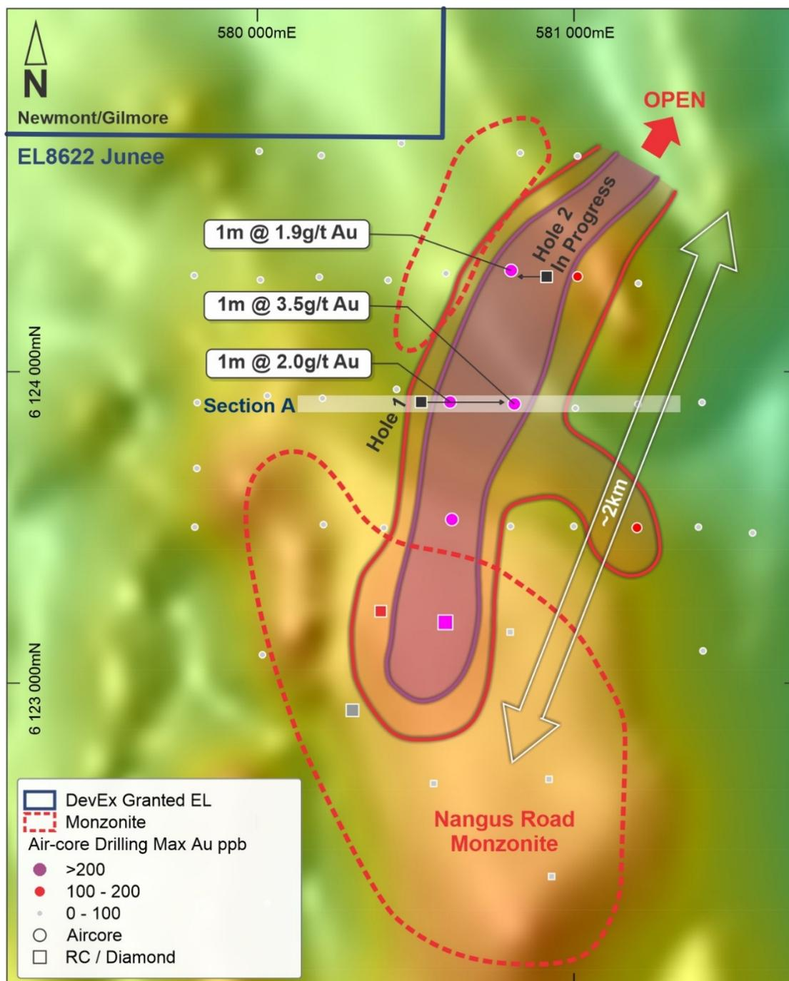
**Figure 2:** Nangus Road Prospect showing location of current diamond drilling 21JNDD001 and 22JNDD002 (Hole 2 - in progress) testing the 2km long bedrock Au-Cu anomaly on 400mN spacing. RC and AC drilling has also commenced and will infill the previous AC intercepts.
