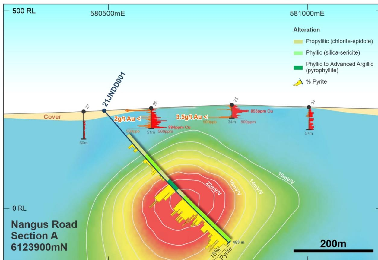
**Figure 1:** Cross section, including modelled 3D IP chargeability anomaly, showing recently completed diamond hole 21JNDD001 which has encountered significant hydrothermal alteration zone down-hole with corresponding visual estimate of pyrite underlying last year’s gold-copper reconnaissance AC intercepts. Assays pending.
