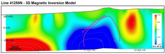
**Figure 2:** Section 41250mN at Billabong Creek Prospect showing buried Inverted Chargeability IP Anomaly (top – red) in close association with the Magnetic Inversion Model magnetic low (bottom – blue).
