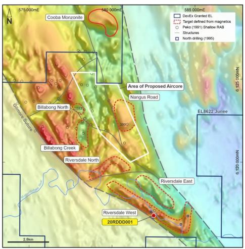
**Figure 4:** Junee Project, NSW, location of Prospects within EL8622, where several porphyry copper-gold targets have been identified based on mapping, historical exploration and interpretation of airborne magnetics (underlay) and gravity.
