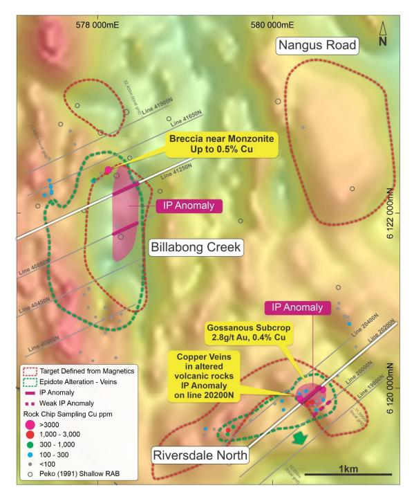
**Figure 3:** Location of recent Chargeability IP Anomalies plotted with the 2019 rock chips at Billabong Creek and Riversdale North. Details of rock chip results are provided in Appendix 1 and reported in ASX Announcement – 11th September 2019.
