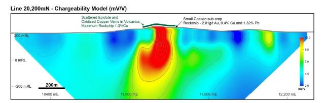
**Figure 1:** Section 20200N at Riversdale North Prospect showing location of chargeability IP anomaly (red) underlying an area of scattered epidote and oxidised copper veins including small gossanous sub-crop (refer to Figure 3, Table 1 and Appendix 1 for detail of the 2019 rock chip sampling).
